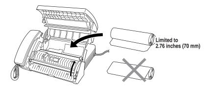
Raise the paper enough to pass it over the  $\sqrt{1}$  until it feeds out the front of the machine. Make sure there is no slack.
